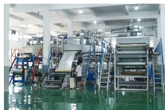
1600#PET保护膜高速涂布机 1000#铝箔高速涂布机 1000#Aluminum High-speed coating machine
