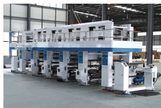
1000#高速凹版印刷机 1000# High-speed gravure print machine
