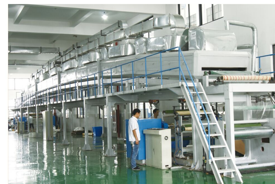
1300型BOPP线棒高速涂布机 1300 BOPP wire rod high-speed coating machine
